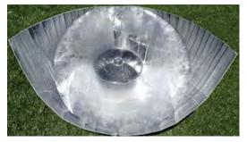
elevates the black cooking pot, eliminating the need for a plastic bag. A second layer of insulation is provided by a circular polycarbonate windscreen, which stabilizes the cooker and creates "oven-like" conditions around the cooking pot. The windscreen also provides extra stability in windy conditions as illustrated in this photo taken in Borrego Springs with 15 mph wind gusts. This solar cooker is currently being sold and evaluated as part of a Rotary San
